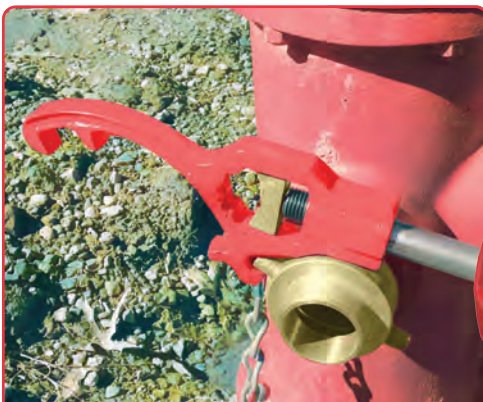
WORKS ON HYDRANT ADAPTERS AND HOSE COUPLINGS, BOTH PIN AND LUG TYPE.
