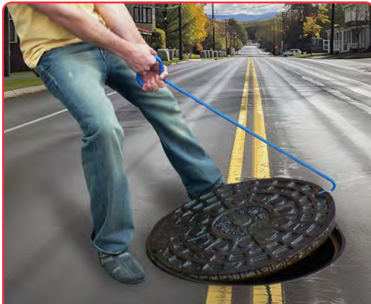
MANHOLE HOOKS ENGAGE PICK HOLES.
