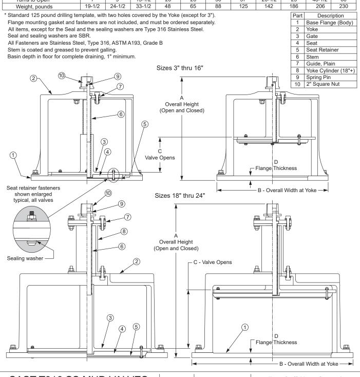
CAST T316 SS MUD VALVES NON-RISING STEM TYPE Drawn to Scale
