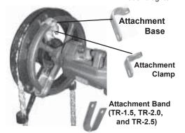
Use Attachment Bases with Clamps (a Band is used in place of one Clamp Assembly on smaller sizes) to secure the Chainwheel to the valve handwheel as shown above. Slots in Chainwheel allow adjustment for range of handwheel diameters; slots in Base and Clamp allow adjustment for various handwheel rim diameters.
