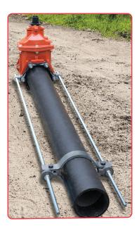
The number of restraining rods required for a specific application must be carefully engineered. The engineer must to take into account factors such as pipe diameter(s), peak pressures, deflections, and other key variables, when determining the correct number of TIE LUGS to be used. Note: The chart to the right shows the minimum number to be used, for sizes up to 16".
