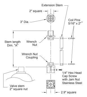
\* Style "A" uses 5/16" x 2" Coil Pins, Stainless Steel Style "B" uses 5/16" x 3" Coil Pins, Stainless Steel
