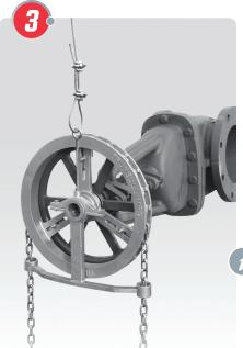
Loop cable through eyebolt leaving about 6" excess.
